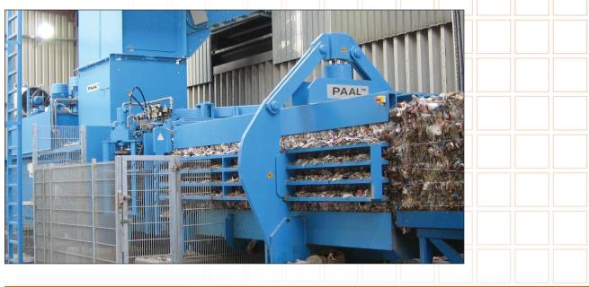
Kadant PAAL's DOKON fully automatic channel baler's unique design makes the PAAL DOKON baler a powerful, efficient bale press with horizontal twine tying system. The PAAL DOKON baler provides a pressing force of 90 to 218 tons and offers a bale format of 32" x 44" or 44" x 44". The combination of high pressing force, independence from the cutting and compressing process, and patented pre-press setting combined with individual channel adjustment lead to high quality baling results.
