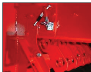
5 Dampened wire guide roller undercarriage
