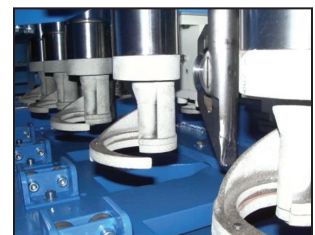
4 Tying system with bolted replaceable wear plates
