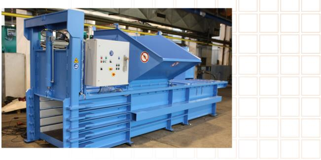
The PAC baler with a vertical sliding door is designed for manual strapping of the bales with wire in a horizontal direction.
